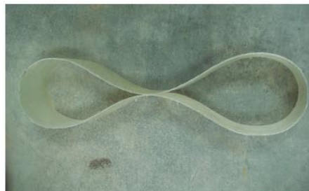
Figure 4. '8' shapped fibreglass developed for tensile test
