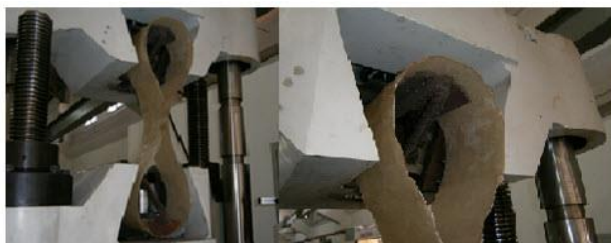
Figure 1. Shimadzu UH-F1000 kN tensile test machine and designed clamps
