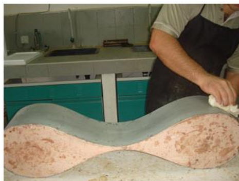
Figure 3. Applying wax on '8' shaped mould
